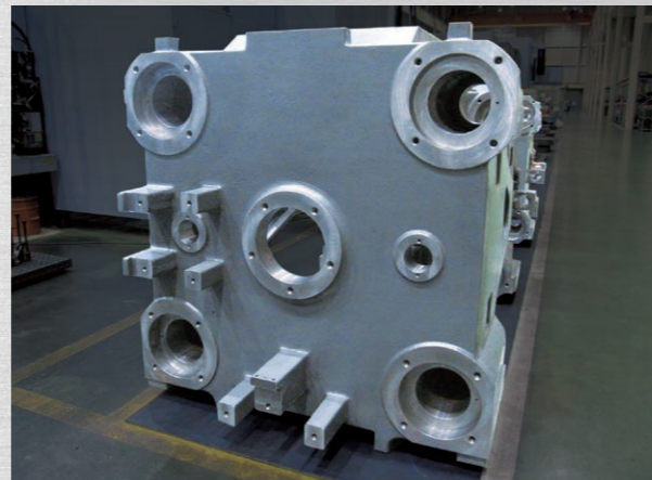
Name: End Plate Material: Casting
